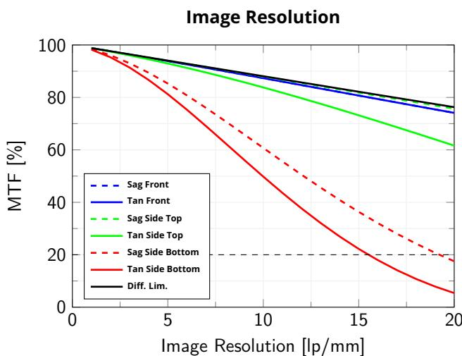
Modulation Transfer Function (MTF) vs. Image Resolution, wavelength range 486 nm - 656 nm of cylindrical object of diameter 20 mm and height of 15 mm, at  $wf/N = 16$
